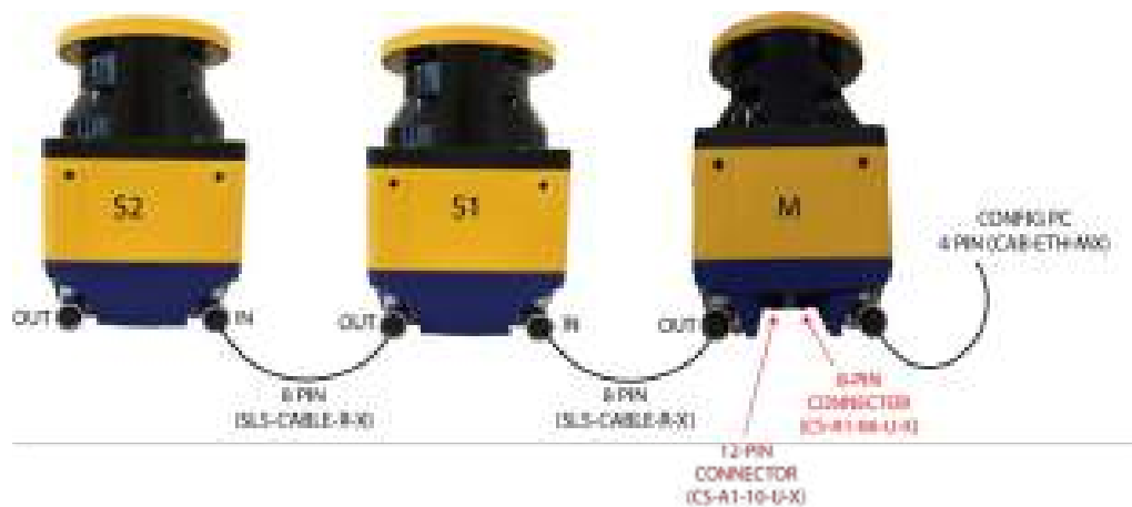
Figure 7 - Master - Slave connection (older software versions)
